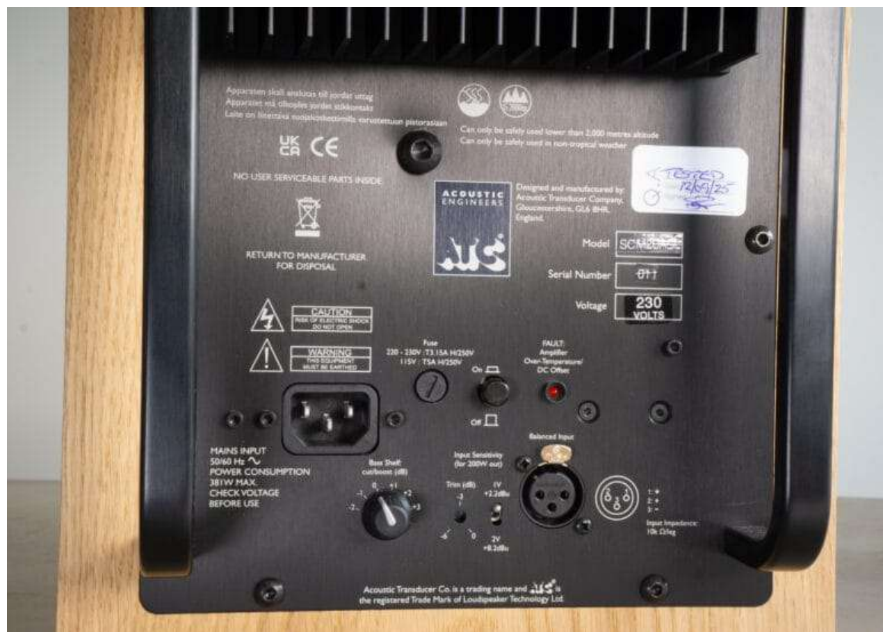
Rear panel inputs and controls with mains and signal input (XLR), power on/off, sensitivity and bass adjustment controls
